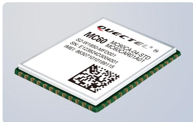
MC60 is a quad-band full-featured GSM/GPRS module using LCC castellation package. With an extensive set of Internet protocols (TCP, UDP, PPP, FTP, HTTP and SSL), it has integrated the GNSS technology for satellite navigation. Based on the latest 2G chipset, it has the optimal performance in SMS & data transmission as well as audio service even in harsh environments. It features Dual SIM Single Standby function.
